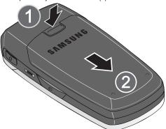
• To remove the battery: pull the top of the battery away from the phone (1) and disconnect it (2).
